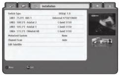
You can select LNB switch type which you are now using. If you choose DiSEqC item, each DiSEqC port assign to LNB by number. In other words, DiSEqC port 1 assign to LNB1 and DiSEqC port 2 assign LNB2 and so on.
