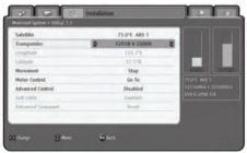
**Step-1.** Select satellite and transponder as you wish to setup. **Step-2.** Move to motor control item and select "Go to" option then press button. The antenna will move to stored position which receiver has.
